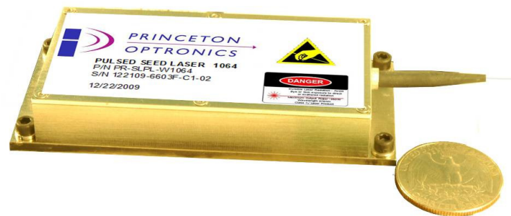
Picture of the seed laser. Package size- 89 x 38 x 15 mm
