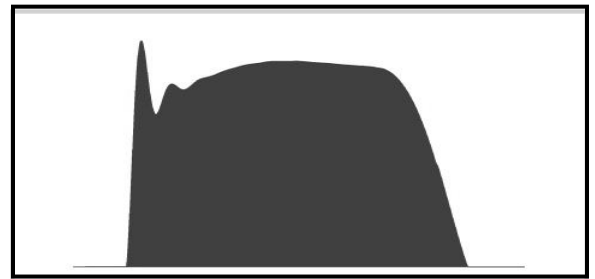
Ideal pulse from a laser driver (2-4 ns)
