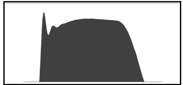
Ideal pulse from a laser driver (4 ns)
